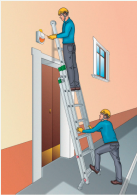
Example of a convertible ladder with three sections in an A-frame configuration supported at the base by another individual.
