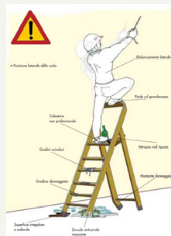
Incorrect usage example: (INAIL technical notebooks - portable ladders)
