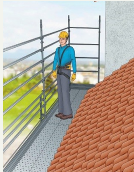
Example of scaffolding utilized for edge protection.
