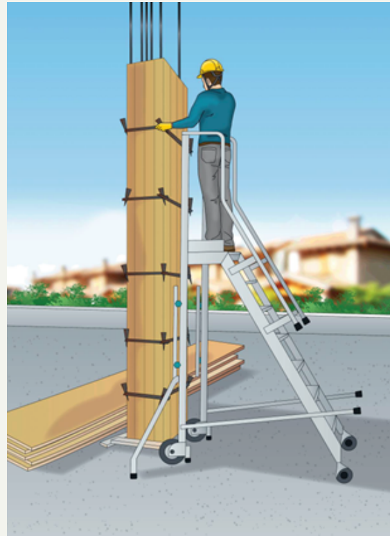
Mobile ladder with platform example, compliant with UNI EN 131-7.
